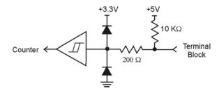
Figure 12. Typical USB-1616HS-2 counter channel
